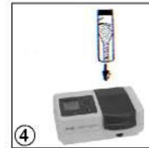
4 measure OD of diluted ciliate suspension at 440 nm
